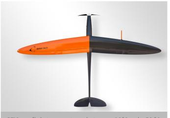
DT18 can fly in temperatures between -20°C and + 50 °C
