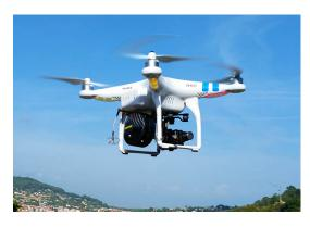
Depending on type of DRS, our systems can safely recover from altitudes around 10 to 15 meters above ground level.
